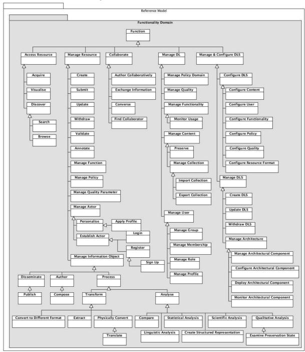
Figure B-5. Functions Hierarchy UML Class Diagram
